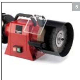
Fixing protective cover
