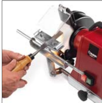
Chisel sharpening attachment
