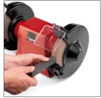
Hand dresser for roughening, correcting and cleaning the grinding wheel
