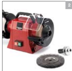
Extension spindle for right-hand side
