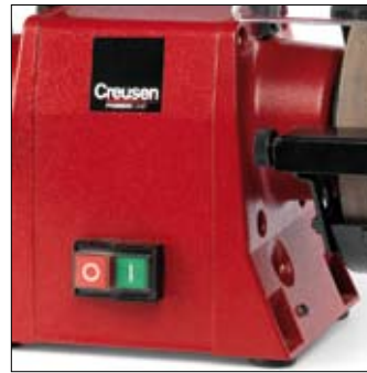
Switch in middle of machine for convenient operation
